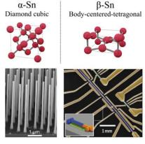
beam epitaxy (MBE) system. In NWs a precise control over the growth of  $\alpha/\beta$ -Sn phases (*i.e.* TOP/SC) becomes possible, resulting in defect-free atomically-sharp interfaces with the highest purity. This will provide a truly *homogeneous integration* of multiple states of matter in solid-state quantum devices, paving the way to explore the fundamental processes in topological quantum computation,(3) spintronics,(4) and quantum photonics.(5)
